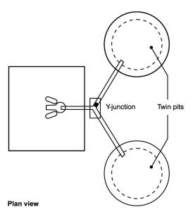
**4.** When the second pit is full, the first pit is emptied. Because the content of the first pit has been maturing while the second pit fills, the excreta has become innocuous — it has lost any unpleasant smell and all pathogens have become inactive. As the pit is small and the sludge is no longer unpleasant or a health risk, the contents can be dug out by the family and neighbours.
