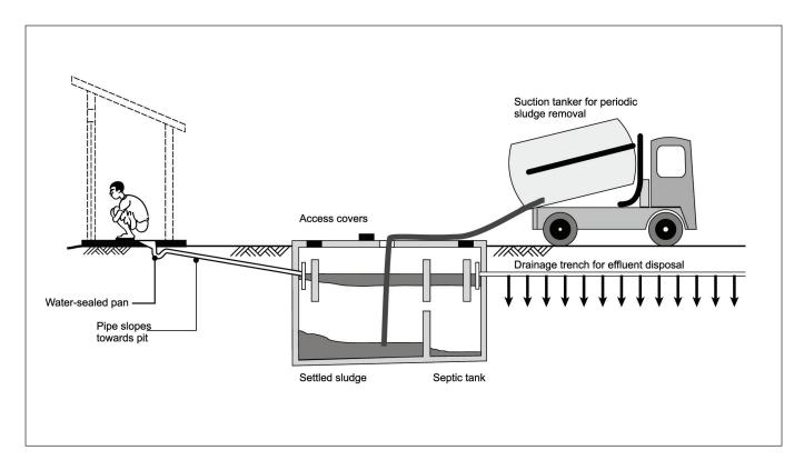
Sludge accumulates at the bottom of the tank. While lying there, it slowly decomposes by anaerobic digestion.
